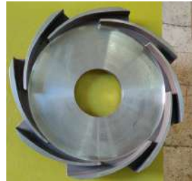
Diffuser in SS410 steel
